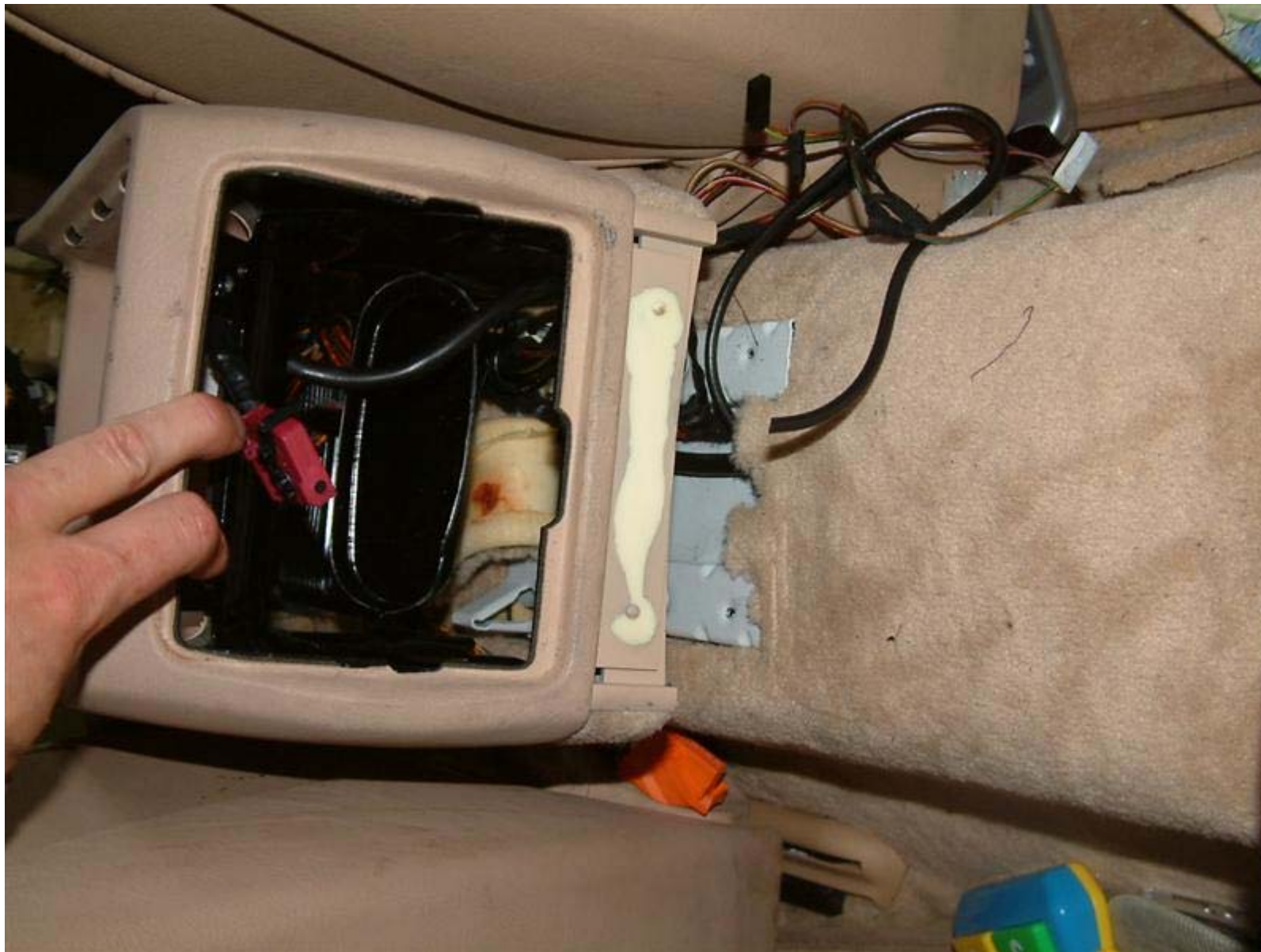
Using this path I was easily able to get the harness up front with plenty of slack
