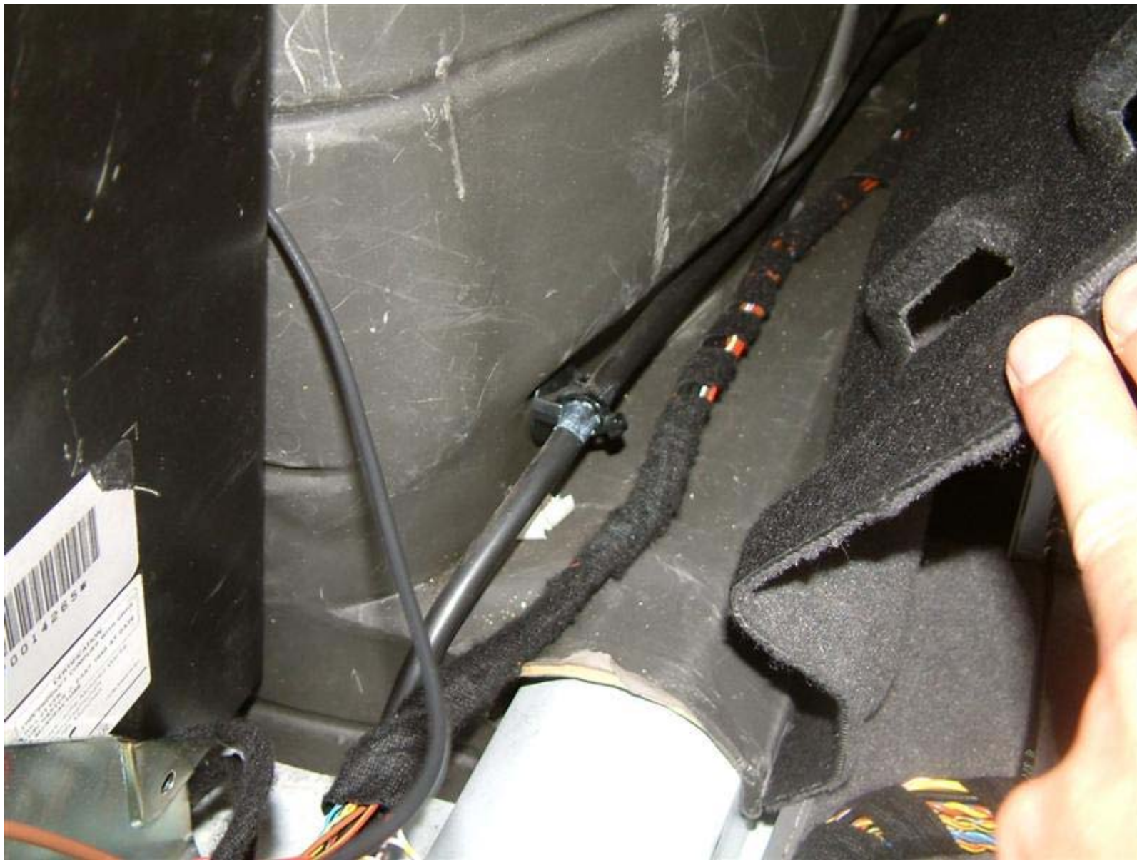
This route leads to just below the rear arm rest where you can find a nice passageway thru. It was hard to photograph, but you can see the black plastic passageway, just at the bottom of the metal and top of the insulation.
